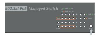
Figure 10-2: GS-4210-8P2T2S Reset Button
