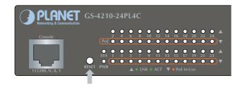
Figure 10-4: GS-4210-24P(L)4C Series Reset Button
