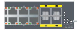
Figure 10-5: GS-4210-48T4S Reset Button
