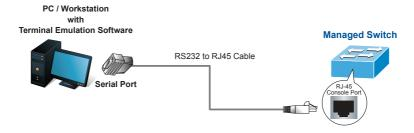
Figure 4-1 Managed Switch Console Connectivity
